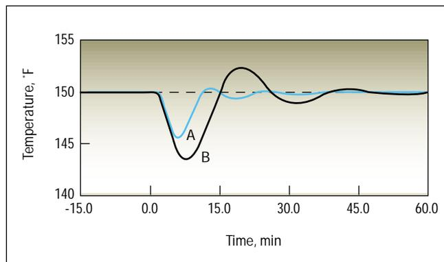
gain of 0.5%/ % and a reset time of 5.0 min gave a critically damped response. Shortening the reset time to 1.8 min, however, gives a response with a quarter decay ratio. Figure 4 illustrates two responses — both have a quarter decay ratio, but the responses certainly are not equivalent.
