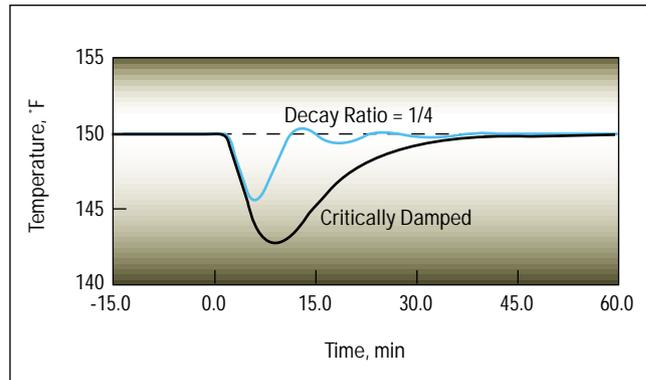
■ Figure 4. Many combinations of coefficients give quarter decay ratio.
